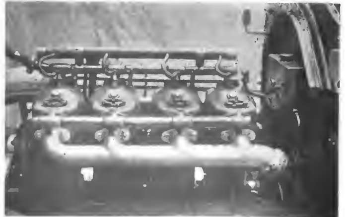
VIEW FROM EXHAUST SIDE OF MOTOR SHOWING OIL RESERVOIR.
